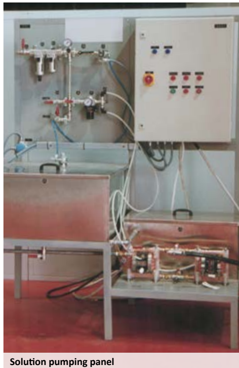
Solution pumping panel
