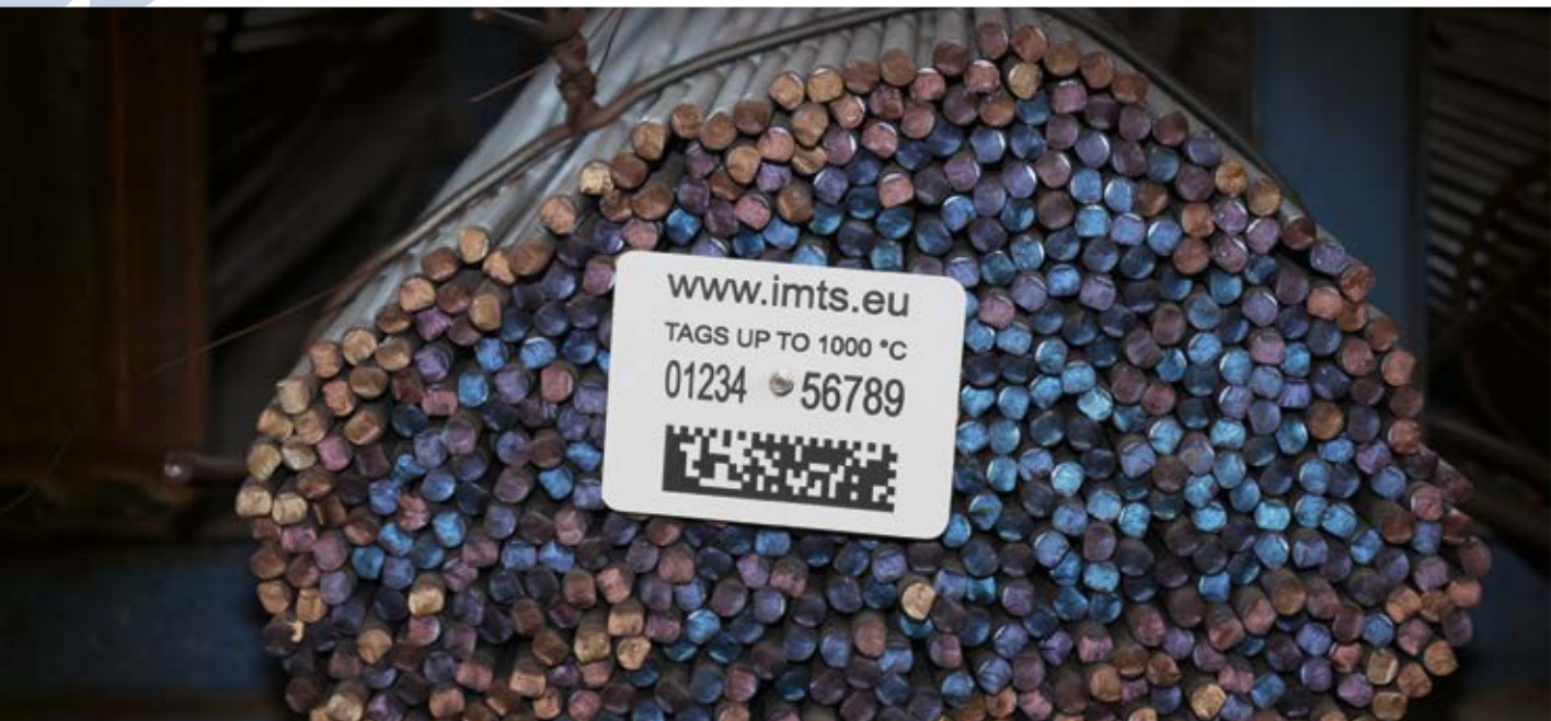
Tag attached by PIN welding
