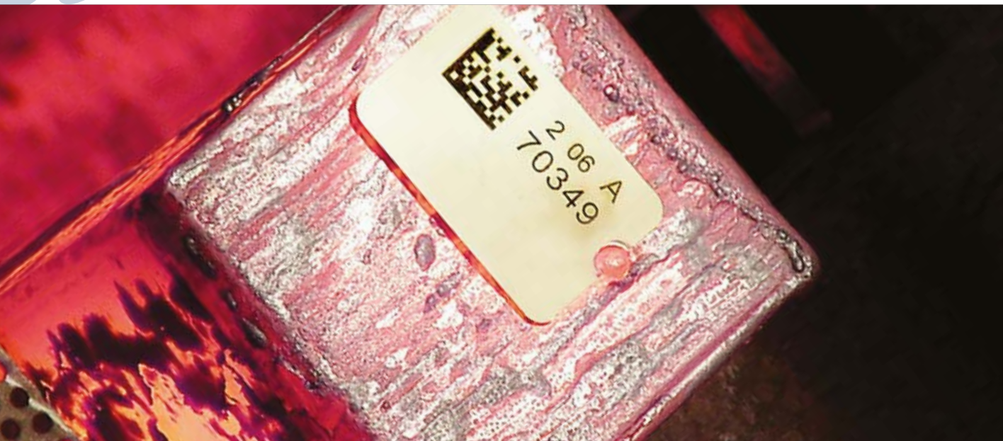
Tag attached by MIG welding
