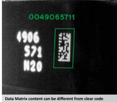
Data Matrix content can be different from clear code
